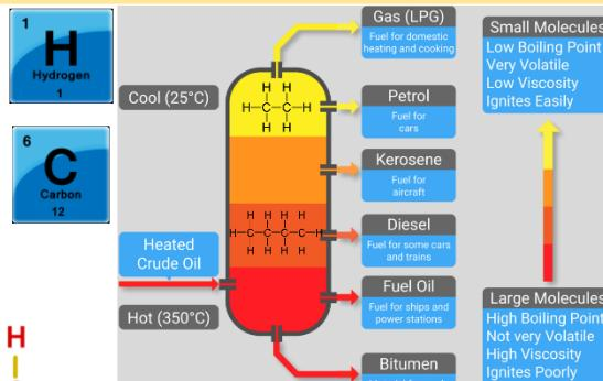
Crude oil is heated and enters the column as vapour. The different compounds have different boiling points, so they condense at different temperatures. The different alkanes separate at different positions in the column. **Fractional distillation**
