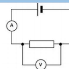
In a **series circuit** the **total resistance** is the **sum** of the resistance of each component.
