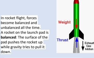
As the engines are ignited, the **thrust** from the rocket unbalances the forces, and the rocket travels upward.
