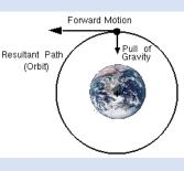
This happens only when the spacecraft is very far from any large **gravity** source such as Earth or the other planets and their moons. If the spacecraft comes near a large body in space, the gravity of that body will **unbalance** the forces and **curve** the path of the spacecraft.
